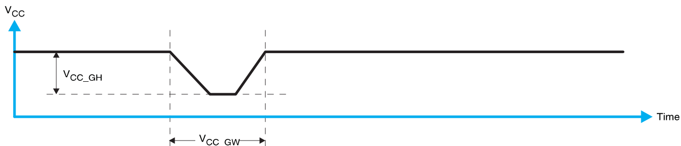
Figure 22. Glitch Width and Glitch Height
